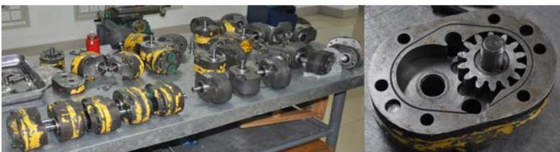
图2 CB-B2.5型齿轮泵
